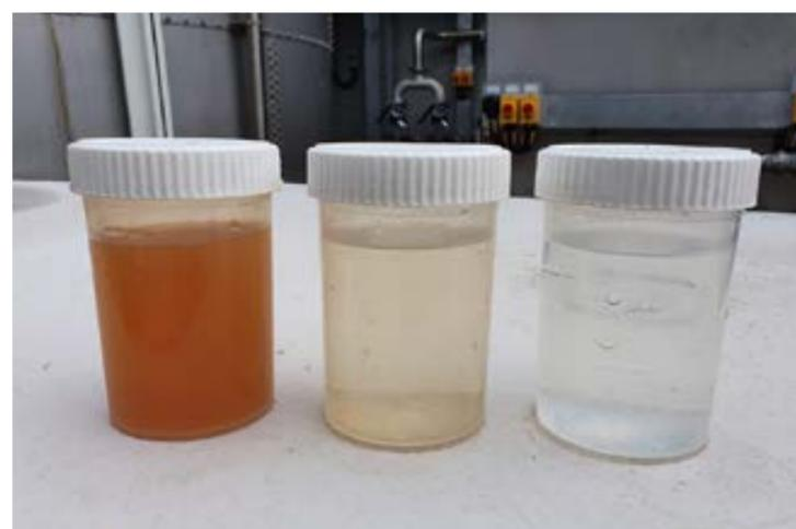
Photo showing (left) raw effluent, (middle) post primary treatment - DAF and (right) post -tertiary treatment - multi-media filtration - AMMF
