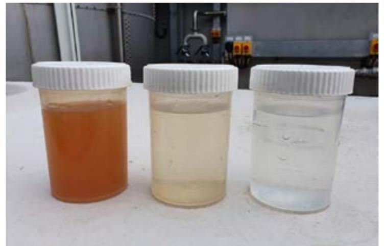
Photo showing (left) raw effluent, (middle) post primary treatment - DAF and (right) post -tertiary treatment - multi-media filtration - AMMF
