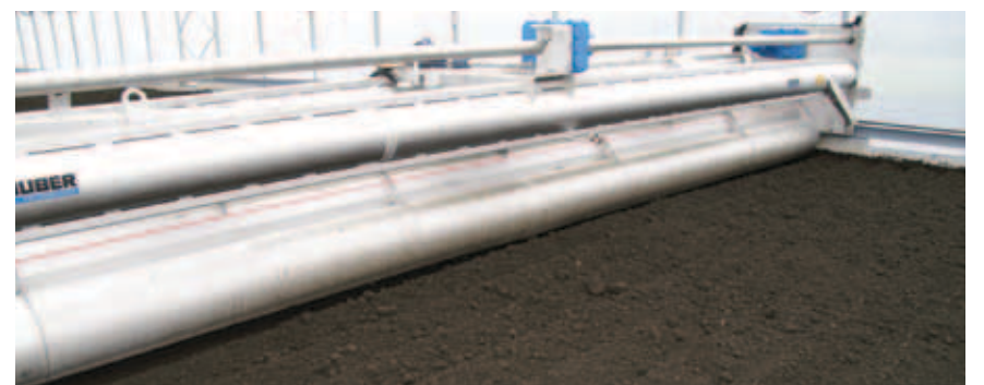
SRT sludge turner installed at a solar drying facility in Germany.
